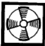
Air vent on panel
